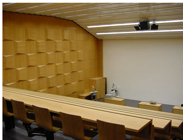
Figure 1: Lecture hall with a central cluster sound system at University of Zurich, Switzerland
