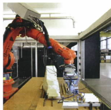
11 Assembly procedure including positioning of insert and welding (Gramazio & Kohler, ETH Zurich, 2014)
